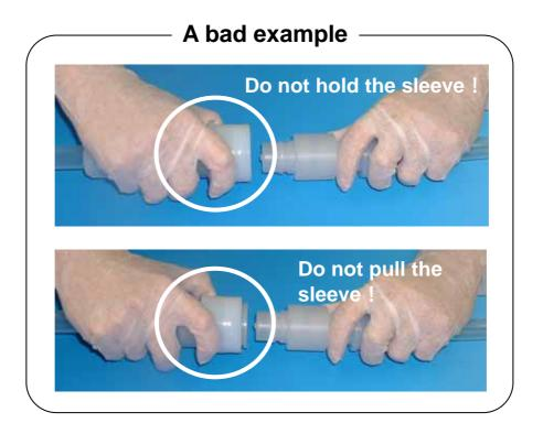
Holding the Saturn ring, insert the socket <u>straight into</u> the plug (See the photo and Figure 2 below).
